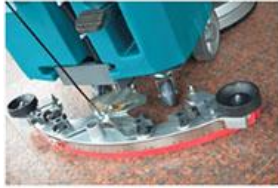
Integrated aluminum die casting water grill, anticorrosion
