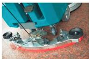
Integrated aluminum die casting water grill, anticorrosion
