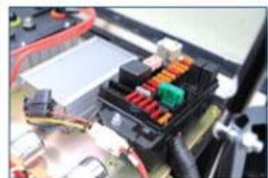
Electric control fuse
