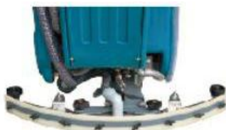
The water sucker can swing with the machine, with fender wheels. It can be fed different hardness sucker stripes.
