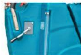
Outlaid clean water level display tube shows the water level clearly.
