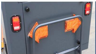
Arrow warning light Rear double arrow warning light, safe operation
