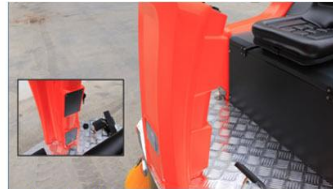
Novel roll front face Two maintenance openings are arranged behind the shell of the rotational plastic steering column, which is easy to maintain
