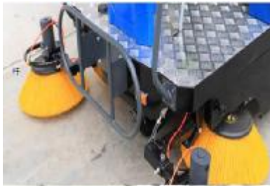
Entrance collision avoidance: The front two-sided brush is equipped with anti-collision circles, and the anti-collision bumper is strengthened in front of the vehicle.
