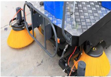
Enhance collision avoidance: The front two-sided brush is equipped with anti-collision circle, and the anti-collision bumper is strengthened in front of the vehicleFront windshiel
