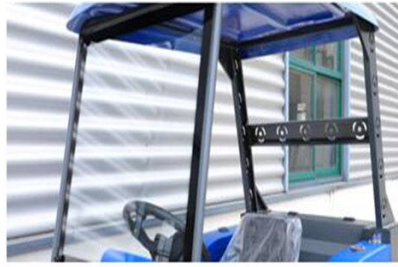
Front windshield: High definition glass on the top of the blister, with higher safety performance
