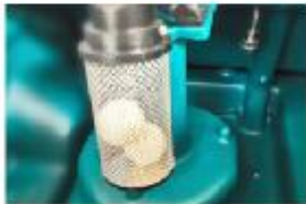
Tank equipped with a water level sensor and will auto stop when the water is full
